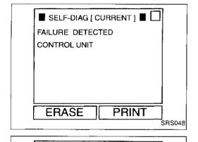
If any problem code was displayed on SELF-DIAG [CURRENT], the malfunctioning part is not repaired completely or another malfunctioning part is detected. Go to DIAGNOSTIC PROCEDURE 2, RS-23, and repair malfunctioning part completely.
